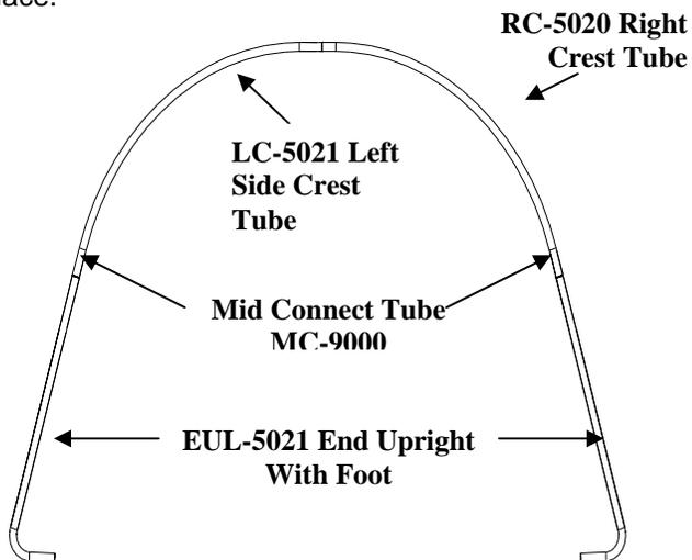
Attach one end upright/mid tube connect sub assembly to each end of a pair to assembled crest tubes to construct each end arch (Qty - 2). Attach one Center Upright/Mid Connect Tube sub-assembly to each side of the remaining Crest Tube pairs to construct the interior arches (Qty - 5).
