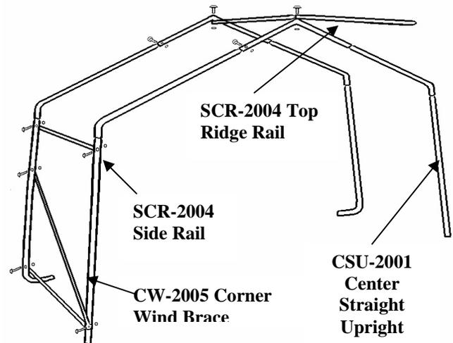
**Step 5.** Begin the Top Ridge Rail by placing a Swedged Cross Rail underneath the End Top Crest Tube. Secure the Cross Rail loosely with a Carriage Bolt#CBN-3000-2 with washer and nut facing the interior of the unit.
