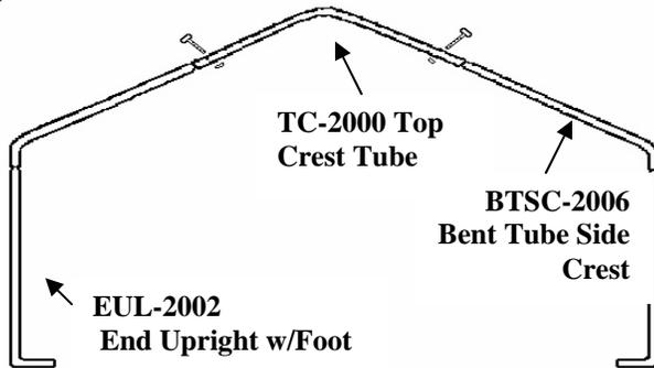
**Step 2.** Assemble the (2) Corner Wind Braces #CW-2005 to the End Upright w/Foot #EUL-2002 to the first of the End Arch assemblies. Use a #CBN-3005-3 Carriage Bolt with Washer and Nut to secure the braces loosely to the Upright. Do not tighten completely.
