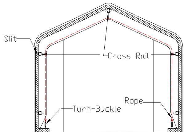
**Note: Adjust/Snug the end panel by turning the turnbuckles or repeating step 3 on a regular basis**
