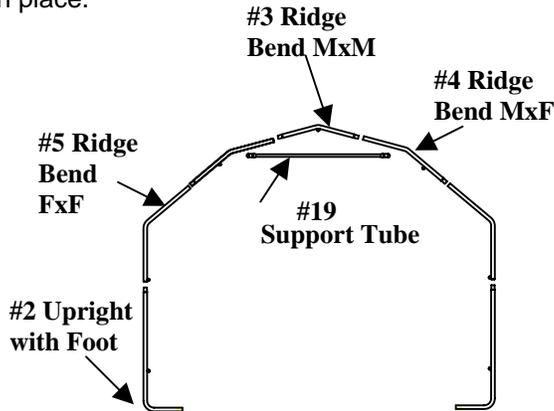
and side hole of the arch upright. Again, don't tighten the hardware until the next arch and cross rails are assembled. It is very important to make certain all nuts are on the inside of the unit to avoid damaging the cover when put on.
